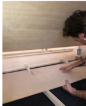
STEP 2: Add first slat and slot in between 'Z' bars.
