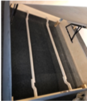
STEP 1: Add two 'Z' bars to the bottom of the frame to support the slats.
