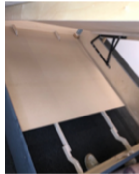
STEP 3: Add the rest of the slats to the bottom of the base. Make sure that they do not overlap.
