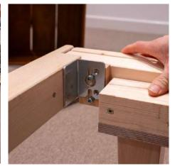
Flip the sides so that the legs are on the floor. Place one side of the footend bracket onto the Hex screws. (The bolts are already in place for you)
