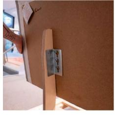
Place the headboard onto the headboard uprights. Using the allen key provided tighten down the bolts.
