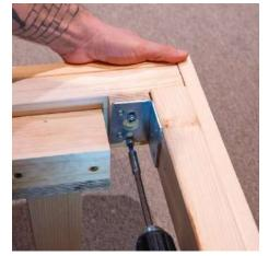
With your other hand make sure that the foot-end and side is flush, whilst screwing the hex bolts down.
