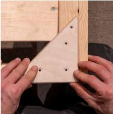
On the head-end place one of the triangles provided flush to the head end and flush to the side as shown in the picture.
