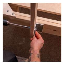
Now using the spanner and allen key provided make sure to tighten the uprights to the bed frame.
