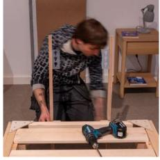
Place the uprights into the bracket at the back of the head-end. make sure that the metal brackets on the uprights are facing inwards.
