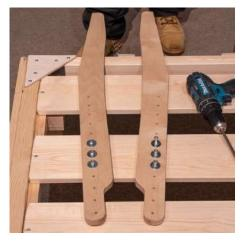
Through the side that doesn't have the metal bracket attached. Place 3x washers and 30mm hex bolts provided through the headboard uprights (starting from the 5<sup>th</sup> hole from the bottom).
