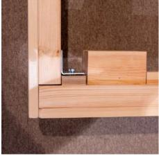
Make sure that the side and foot-end is flush to each other. Screw in the hex bolts with the allen key provided to tighten to the metal bracket. Making sure its all flush.
